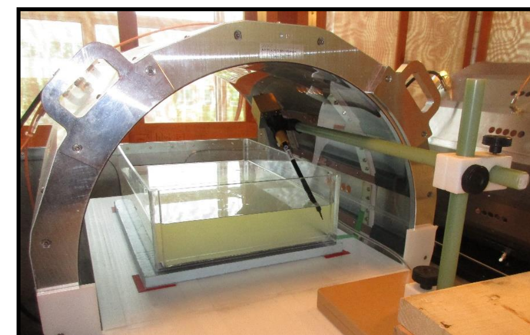
Figure 3: Representative measurement setup using a calibrated EASY4 E-field RMS probe in the MITS 3.0.
